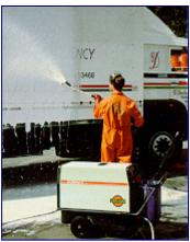
After coating the vehicle with foam the dirt is absorbed immediately by the foam and removed ensuring optimum contact between the detergent and the vehicle. This foam film is quite naturally very easy to rinse off. After drying a gleaming surface emerges that makes the vehicle less prone to retain dirt.
